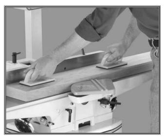
Figure 36. This is an example of a surface planing operation.
